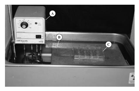
Fig. 3 Water bath used to perform the postendocytic fate assay. The water bath is equipped with a temperature regulator/circulator (A). A  $22.5 \times 26$  cm aluminum plate (B) is placed on top of test tube racks, and the water in the bath is adjusted so that the aluminum plate is covered by approx 5 mm H<sub>2</sub>O. A 12-well plate containing Transwell filters (C) is placed on top of the aluminum plate.
