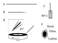
**Fig. 1** Carbon fiber microelectrode construction following Wightman's method (see text).
