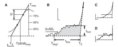
**Fig. 4** Determination of spike (**A**) rising phase parameters and (**B**) PSF characteristics. Examples of PSF without (**C**) and with (**D**) detectable steady states. Horizontal lines indicate  $I_{foot}$ , which equals average (**C**) or steady-state (**D**) currents within  $t_{foot}$ . Dashed lines represent spike baselines. Bars = 10 pA and 1 ms.
