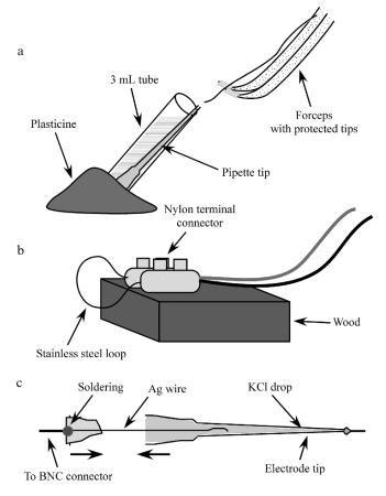
Fig. 3 Electrode construction using pipet tips (explanation in the text).
