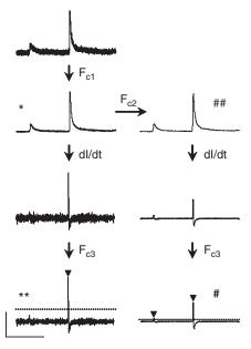
**Fig. 6** The cutoffs of the low-pass Gaussian filters are  $F_{cl}$ , 600 Hz;  $F_{c2}$ , 150 Hz;  $F_{c3}$ , 300 Hz.  $F_{sp}(max)$  is approx 300 Hz. Arrowheads on the bottom panels denote spikes that exceed  $5 \times SD_{dl/dt}$  (dotted lines). Bars = 20 pA, 10 pA/ms, and 100 ms.
