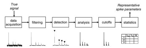
**Fig. 1** An overview of amperometric data acquisition and analysis. The original "true" amperometric signal is ultimately represented by spike characteristics analyzed and pooled from multiple recordings. Each analytical step may introduce some degree of signal distortion, depending on the internal characteristics of the recording (signal frequencies, noise level, etc.) and on user-defined parameters of data acquisition and analysis (filtering, detection thresholds, cutoffs, etc.).
