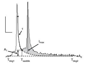
**Fig. 5** Analysis of overlapping spikes. The baseline of the second spike is approximated using exponential fit constants of the falling phase of the first spike. The trace was generated by summing two identical recordings, one of which was offset by 15 ms; the first and second spikes are therefore identical. Dashed lines represent spike baselines; shaded area is an amperometric charge of the second spike. Bars = 50 pA and 10 ms.
